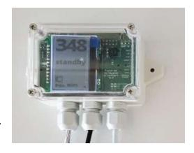
The fully waterproof computer case includes a printed circuit board integrating the LCD display, the IMU, the UART interface to the motor controller, an NMEA0183 port with galvanically isolated input, EMC surge protections and a GPIO connector allowing the use of a Raspberry Pi Zero 2W or Zero W. The printed circuit board is marinized on the component side by applying three layers of tropicalizing varnish.
